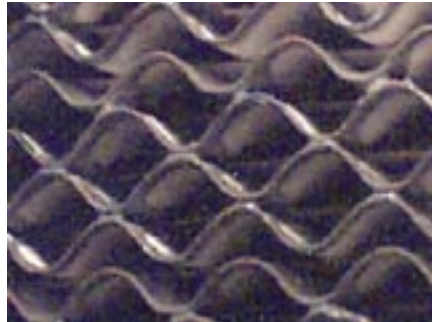
Figure 7: Media shown with anti-stick face coating prior to challenge with heavy ETS in test chamber.
