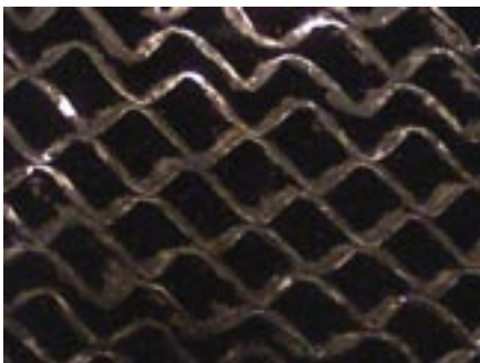
Figure 5: Ten times magnification of core 1, the untreated sample after the simulated 4 years of heavy ETS loading and compressed air cleaning. As compared to Figure 3, much of the buildup has been removed but approximately 30% still remains.
